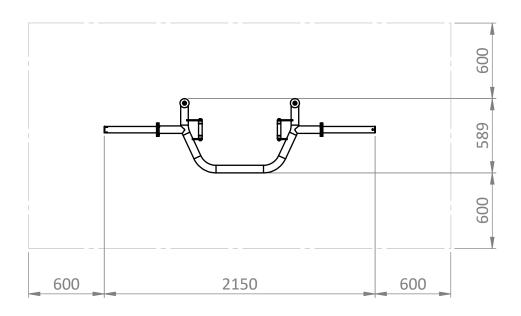
Add sufficient clearance, not less than 0,6 m, on all sides.
