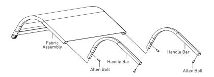
**Step 2**Insert Fabric Assembly into Handle Bar Assembly, and screw the Allen
