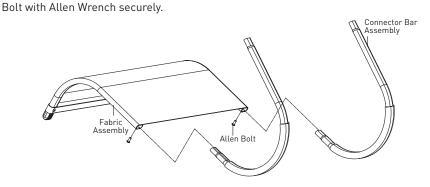
**Step 3**Insert Connector Bar Assembly into Handle Bar Assembly, and screw the Allen Bolt with Allen Wrench securely.
